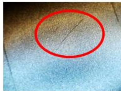
A long, narrow sharp cornered impression caused by movement of a sharp object across a surface
