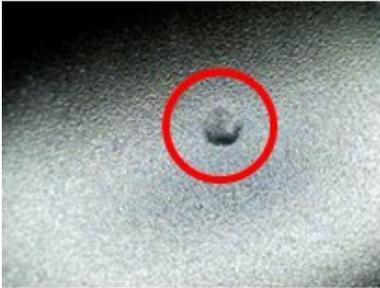
A depression with rounded edges caused by impact with a blunt object
