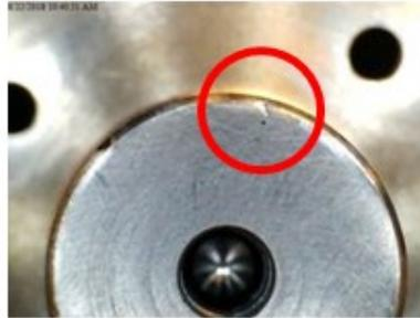
A depression with raised material caused by impact with a sharp edge
