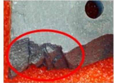
A breaking away of an edge caused by impact from a foreign object
